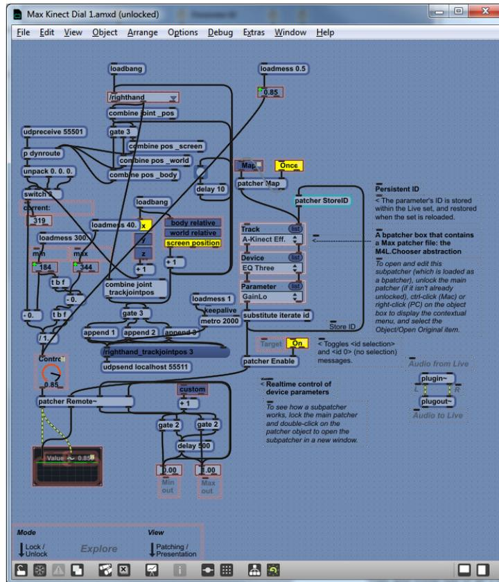
Figure 19. Max Kinect Dial 1 patch, originally taken from Synapse and edited
