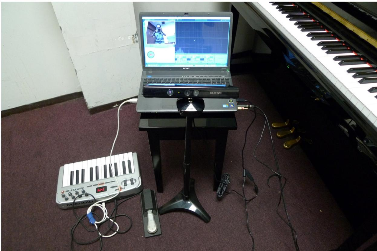
Figure 5. Kinect/EQ Interface hardware setup
