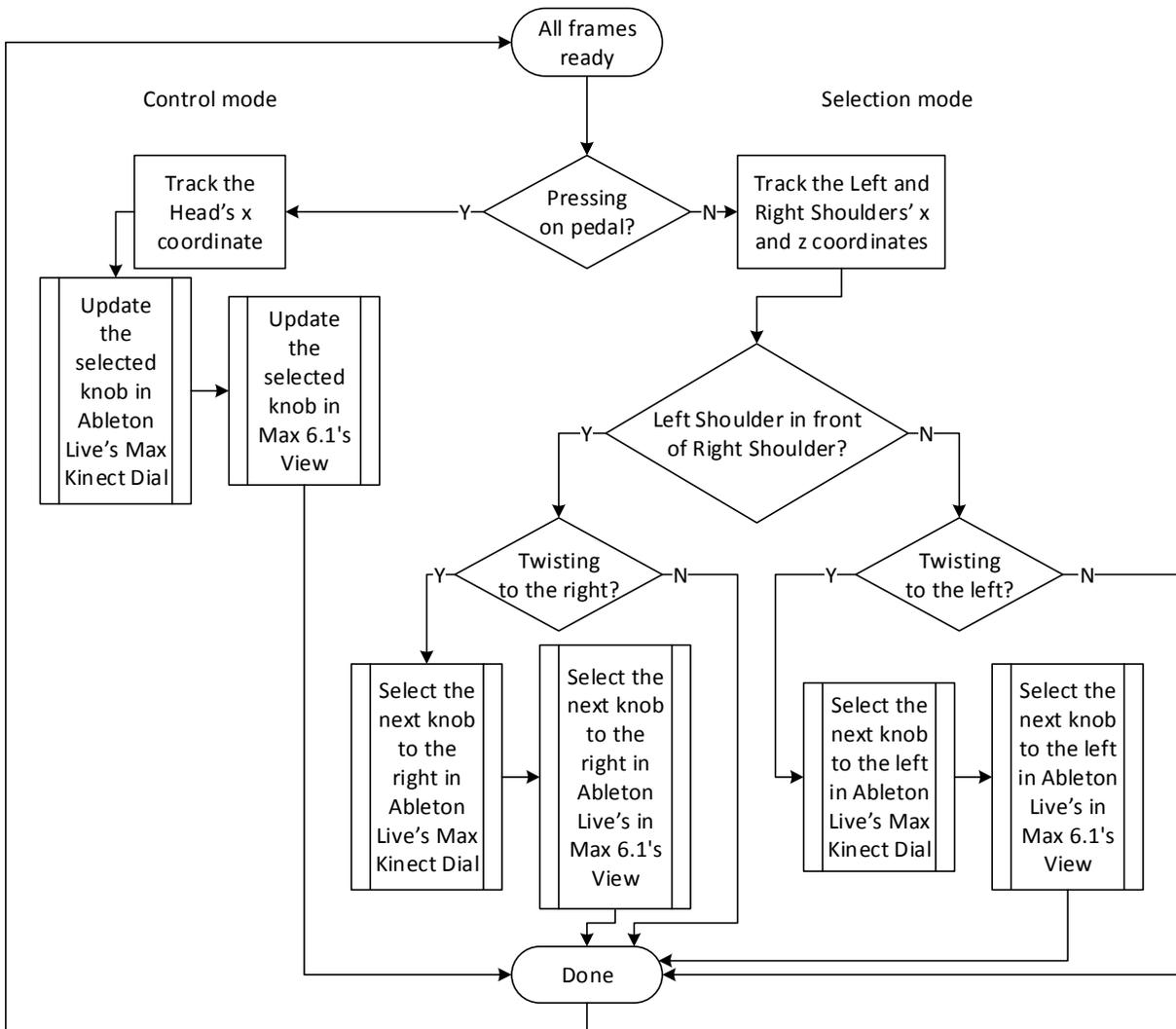
Figure 9. SkeletalTracking.exe workflow when all frames are ready
