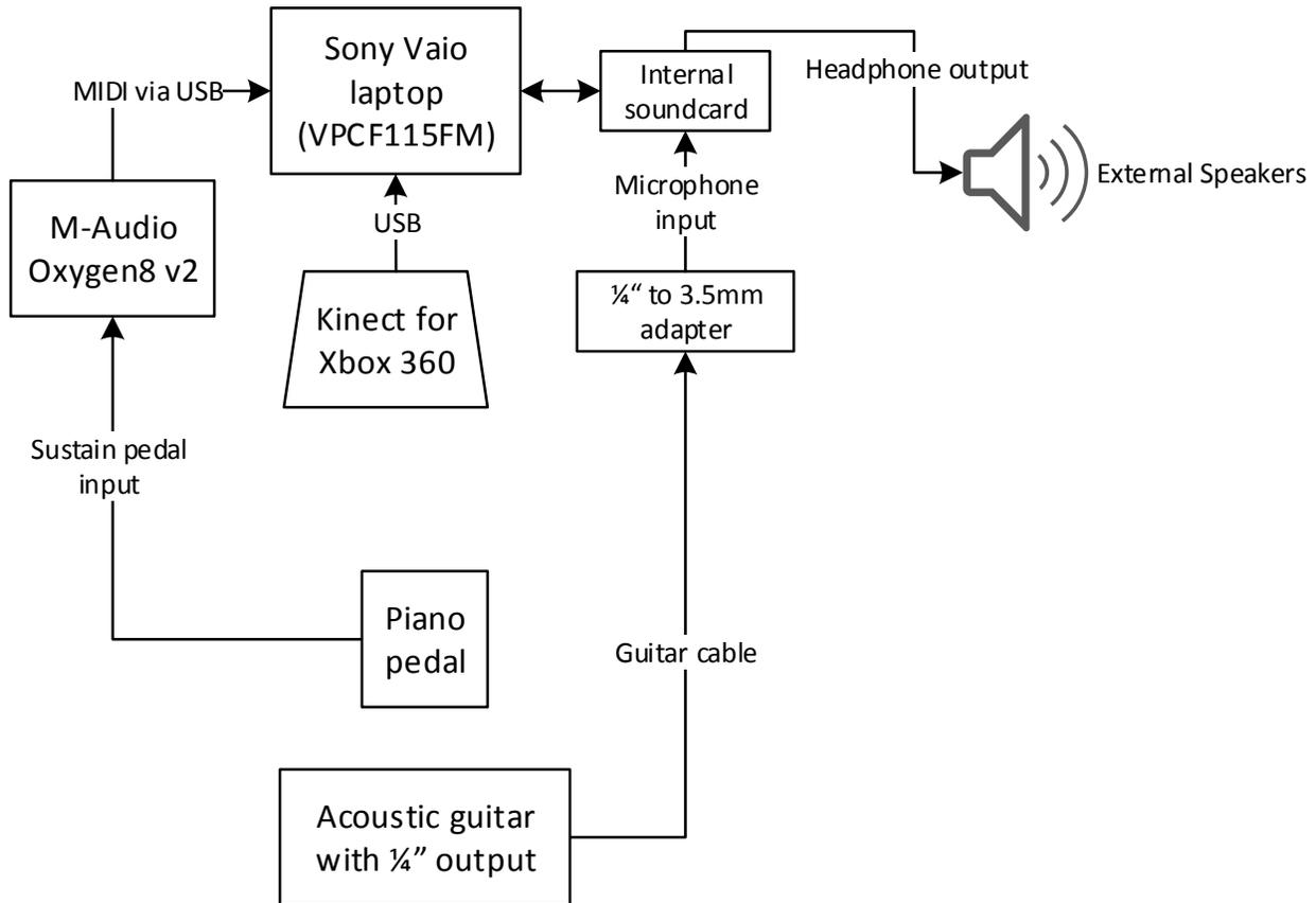
Figure 6. Kinect/EQ Interface signal flow
