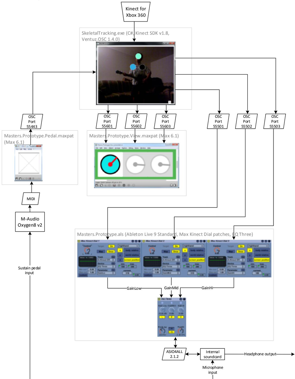
Figure 7. Kinect EQ/Interface architecture
